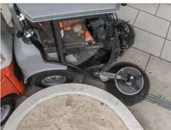
Gets in almost every corner: The steering system with articulated joint ensures excellent manoeuvrability – even when sweeping in reverse gear.
